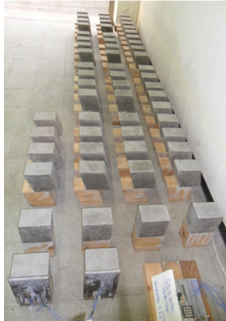
Fig. 5. Specimens on curing.
