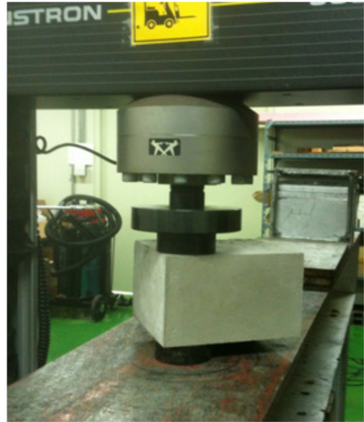
Fig. 2. Compression test of concrete.
