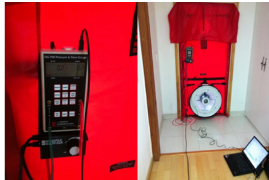
Fig. 3. Picture of equipment for blower door test (Minneapolis Blower Door Model 3, The Energy Conservatory co. Ltd.).
