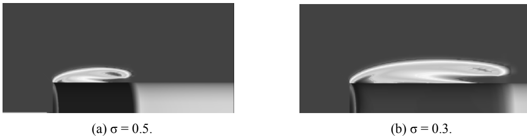
Fig. 10 Liquid volume fraction of 0-caliber cylinder at two cavitation numbers.
