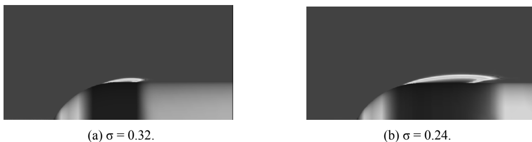
Fig. 8 Liquid volume fraction and surface pressure distribution of 1-caliber cylinder at two cavitation numbers.
