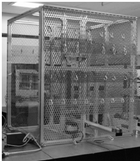
Fig. 6 Structural frame and protection wire-mesh built on heavy surface plate for dynamic buckling tests.
