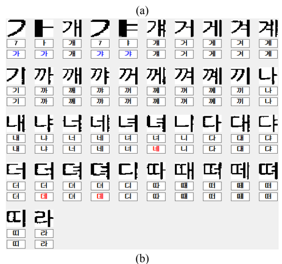
Fig. 16. A sample result of the character labeling method, (a) the detected ROI and the segmented result and (b) the labeling result
