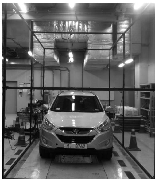
Fig. 3 Photo of hydrogen leakage test system
