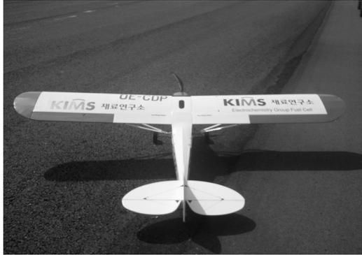
Fig. 14 Fuel cell powered UAV (Super cub 1/4 scale)
