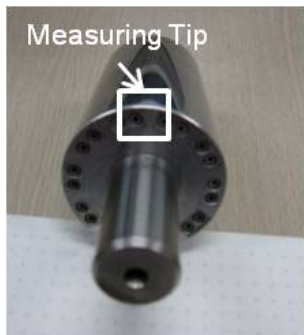
(b) Real cylindrical mold having clamped measuring tip using bolt
