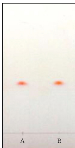
Fig. 1. The thin layer chromatography of hydrolysate of purified \gamma -PGA. A: authentic glutamic acid, B: hydrolysate of purified \gamma -PGA.
