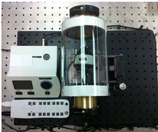
Fig. 1 Experimental set up for roll type photolithography
