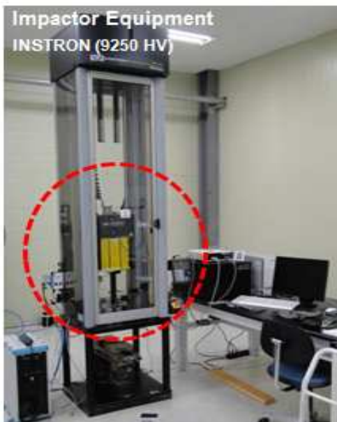
Fig. 3 Configuration of impact test equipment
