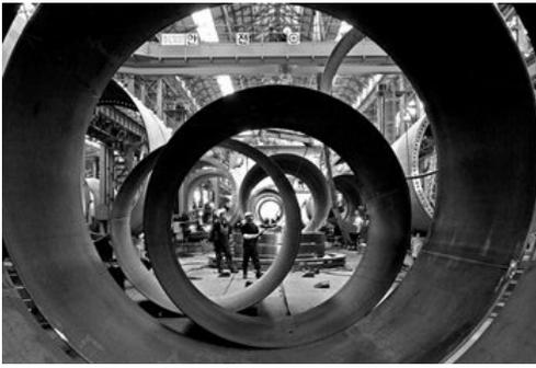
Fig. 1 Manufacturing of tower (Unison)
