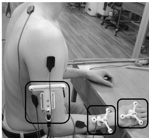
Fig. 1. Positions of the triple active markers attached on the upper limb during eight flower arrangement tasks.
