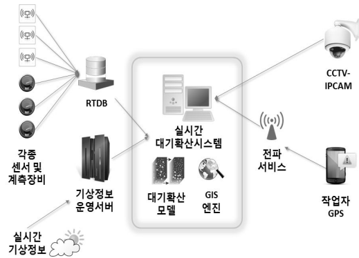
Fig. 5. Real-time Atmospheric Dispersion System Architecture
