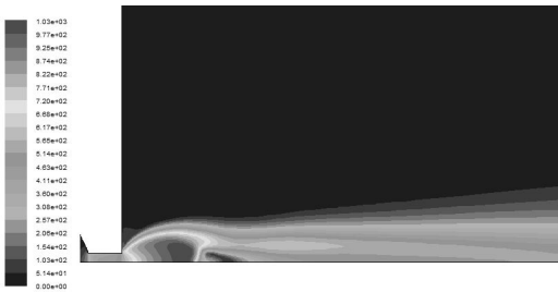
Fig. 4. Velocity profile with 35 bar supply pressure at the nozzle exit(unit : m/s).
