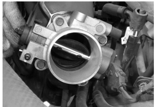
Fig. 7. Carbon deposit of throttle body inside.
