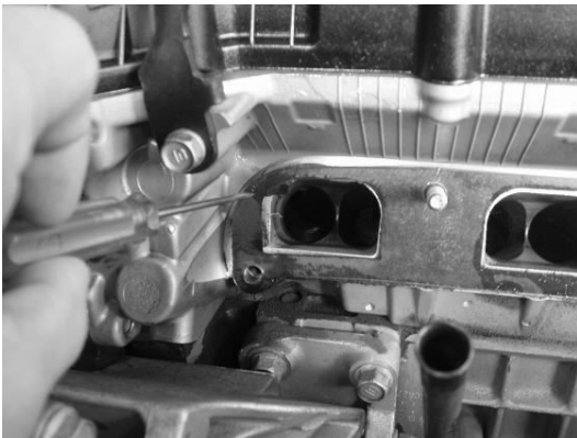
Fig. 8. Damage of intake manifold gasket.
