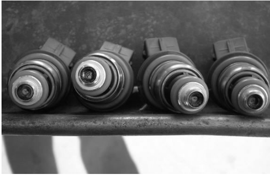
Fig. 5. Clogging example of injector.
