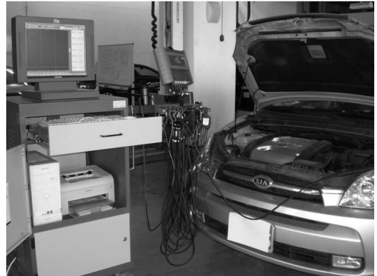
Fig. 3. Engine tune-up tester for pulse form on vehicle engine room.
