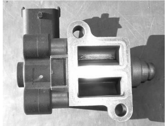
Fig. 6. Carbon deposit of ISA.
