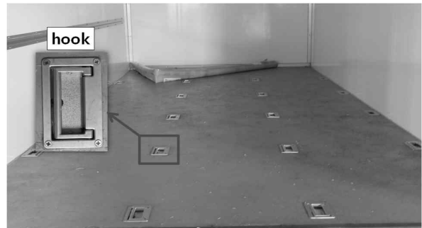
Fig. 10. Hooks for fixing of cargo box
