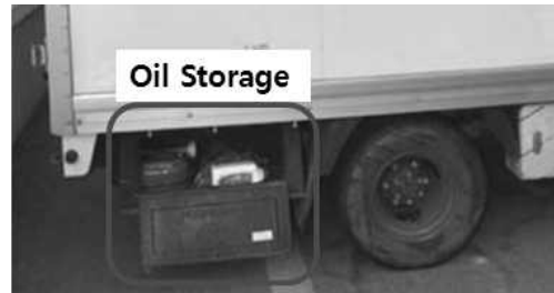
Fig. 17. Oil storage (Fuel, Engine Oil)
