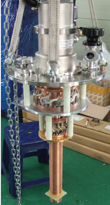
Fig. 2. Internal view of cryogenic vessel for conduction cooling superconductor bulk.
