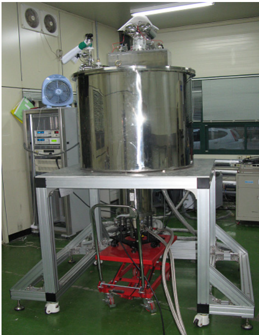
Fig. 5. Magnetization view of cryogenic vessel attached six YBCO bulk by 4 T-class superconductor magnetizer.
