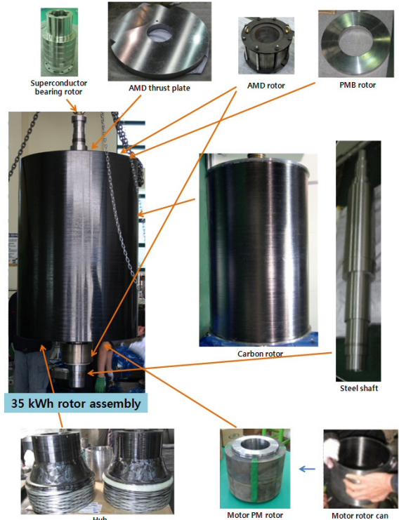
Fig. 4. Major components of 35 kWh class rotor.
