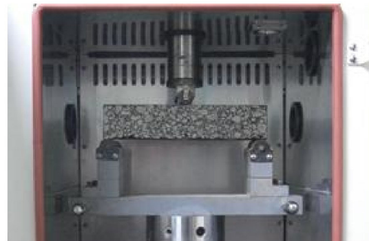
Fig. 6 3-Point Bending Test Setup
