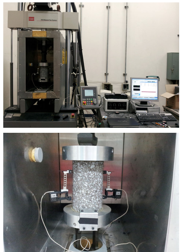
Fig. 8 MTS 810 System and the Setup for Dynamic Modulus Test
