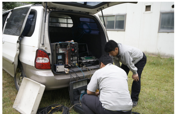
Fig. 4 Producing of Warm Mix Asphalt and Measurement of Emission Gas
