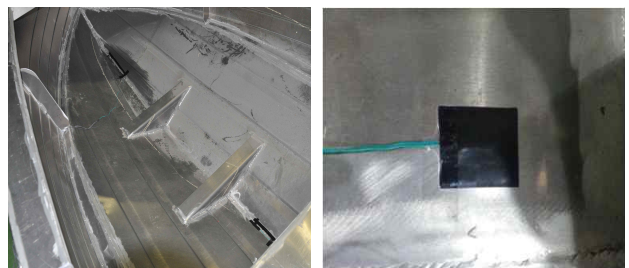
Fig. 4. Pressure and strain-gauge for drop test
