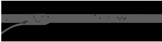
<Figure 5> Location of conflicts in a weaving area: triangle (conflict of rear-end), rectangle (conflict of lane-change)
