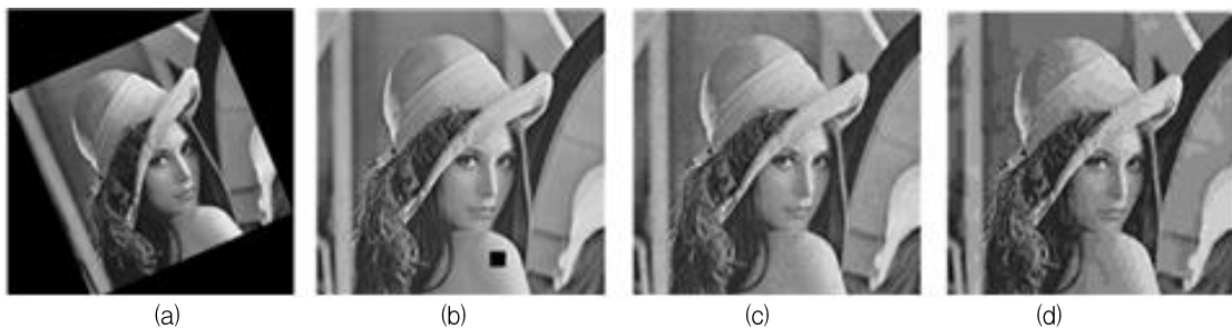
Fig. 7. An attacked images by various image processing. (a) Rotation ( \alpha=10^\circ ), (b) Cropping (50 sub-blocks), (c) Gaussian noise (dev.=2), (d) JPEG compression (r=10).
