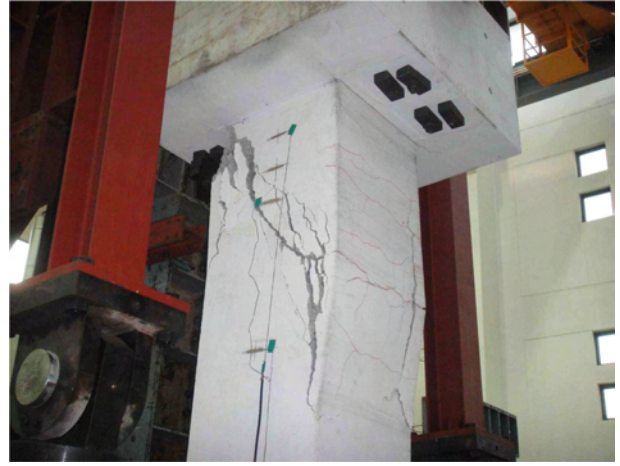
Fig. 4 Final failure of RC
