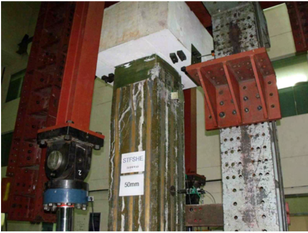
Fig. 6 Final failure of STFSHE
