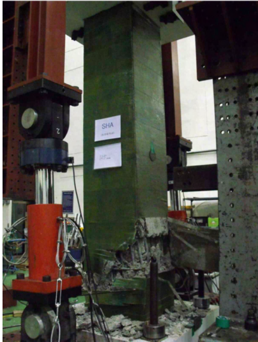
Fig. 10 Final failure of SHA
