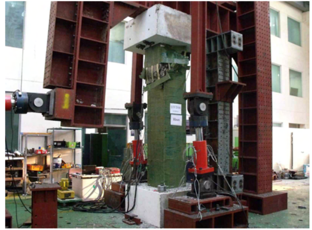
Fig. 8 Final failure of STFSHA
