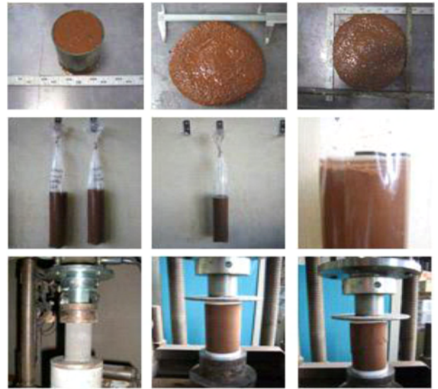
Fig. 2 Flow, bleeding and strength test method
