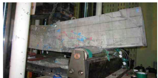
Fig. 6 Shear compression failure
