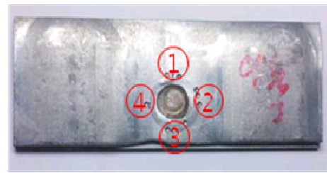
Fig. 1 Spot welding specimen
