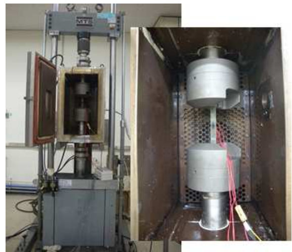
Fig. 2 Photographs for tensile testing system with environmental chamber
