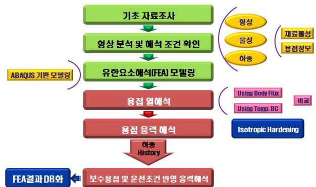
Fig. 5 Scheme of stress analysis
