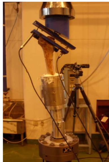
Fig. 10 Stability test scene for hip-joint implant system
