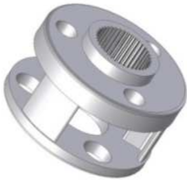
Fig. 2 Configuration of straddle mounted carrier
