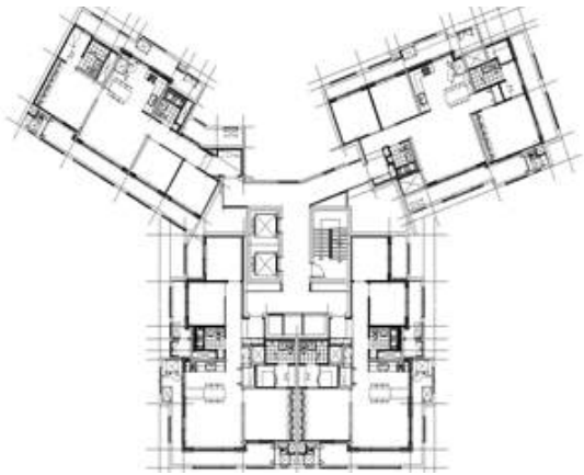
Figure 6. Typical floor plan of bearing wall structure
