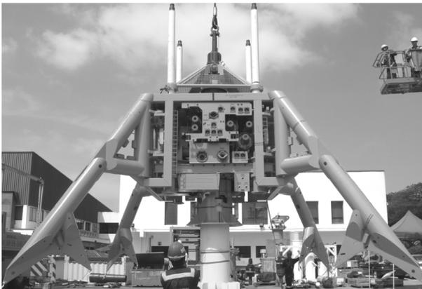
Fig. 10 X-Tree FFS deployed configuration
