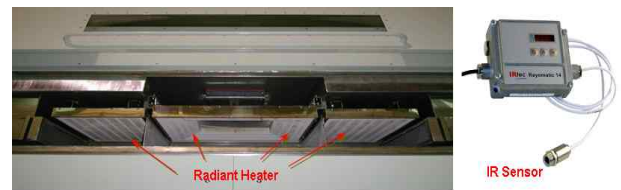
Fig. 3 Radiant heater for powder preheating and IR sensor
