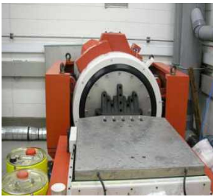
Fig. 6 The vibration test
