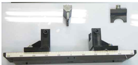
Fig. 1 The bending device for circle tube
