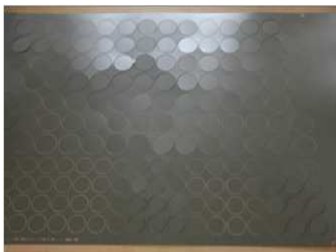
(a) etched stainless steel sheet ( t_m = 50 \mu\text{m} )
