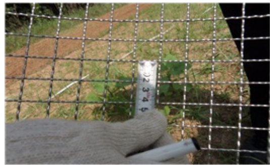
Figure 5. A sieve used for separating soil particles smaller than 20 mm in diameter.
