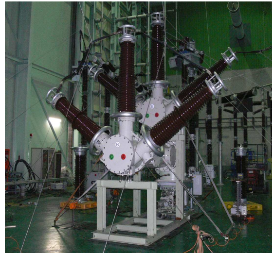
Fig. 9. Test breaker after three-phase synthetic making test
