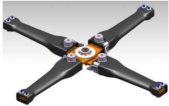
Fig. 2. The Designed Bearingless Rotor Hub
