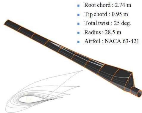
Fig. 2. Aerodynamic configuration design result of 1 MW class wind turbine blade
