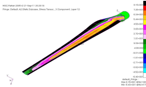
Fig. 10. Spanwise stress contour on spar (21 th ply)
