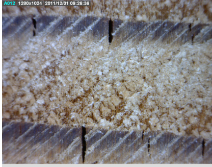
Fig. 5. A microscopic photo of a cross section of a Japanese larch specimen after organosolv pretreatment.
