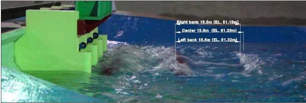
Fig. 11. Flow Shape with 2 Rows of Baffle Block
