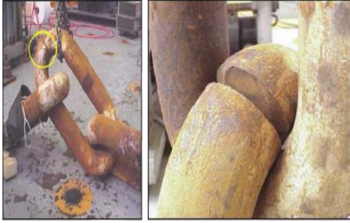
Fig. 3.2: Fatigued sections of mooring chain.
