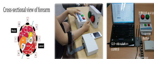
Fig. 2 Attached area of vibrotactile motor (left), experimental position (middle) and experimental system for sensory perception test using vibrotactile actuator (right)
