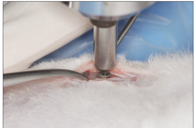
Fig. 3. A photograph of the removal torque test holding the sample. The driver is connected to the implant and the jaws of the digital torque gauge (Mark-10, USA).
