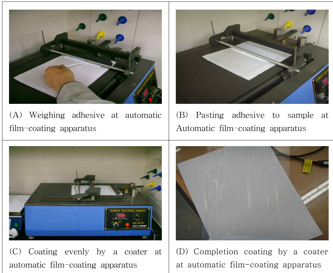
Figure 1. Coating process of tape for repairing archival document.
