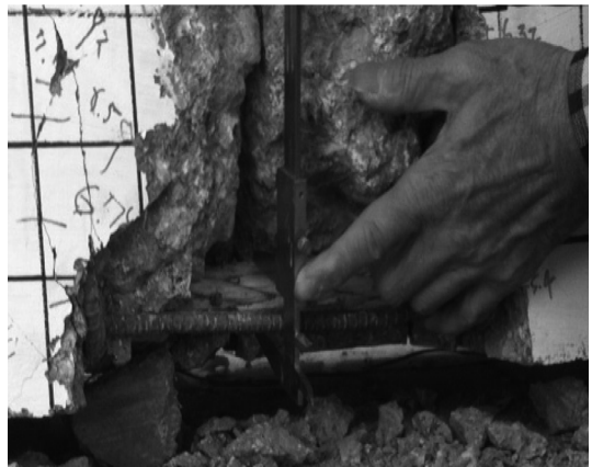
Fig. 10. Super fiber rope in concrete.
