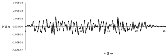
Fig. 8. Displacement time history at the top of structure with centered pivot-type displacement amplification damper system(C = 160,000 kgf · sec/m).
