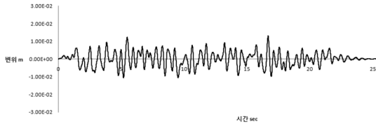
Fig. 9. Displacement time history at the top of structure with distributed pivot-type displacement amplification damper system(C = 80,000 kgf · sec/m).
